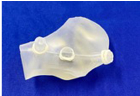
Fig. 6 The final template 3D printed. They are composed of biocompatible photopolymer resin
