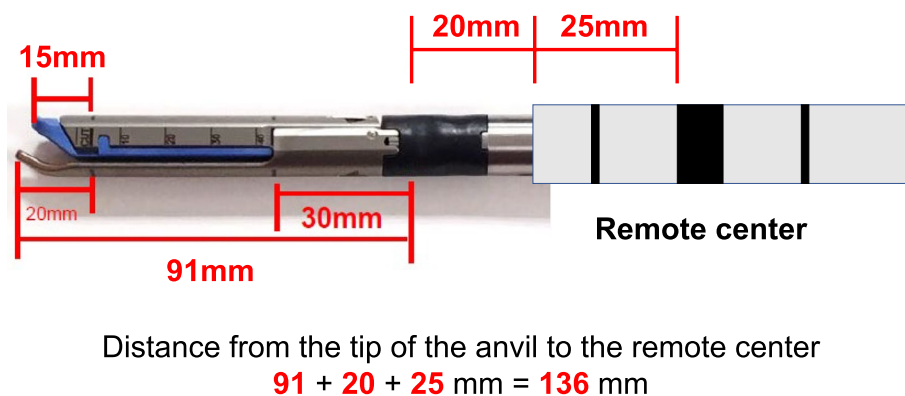
Fig. 3 The SureForm 45 Curved-Tip specification
